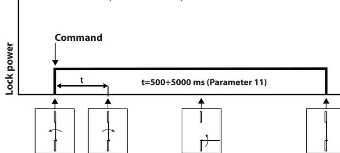
**LOCK WITH RELOCK WHEN POWER IS CUT OFF (Parameter 10=5)**
