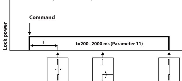
**MOTORIZED LOCK (Parameter 10=4)**
